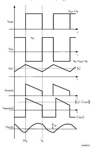
**FIGURE 3. Typical Waveforms**
