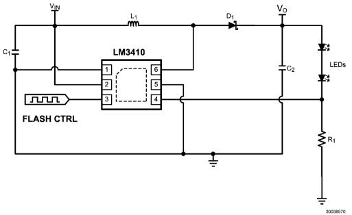
LM3410X (1.6MHz):  $V_{IN}$  = 2.7V to 5.5V, ( $V_{OUT}$   $\stackrel{\text{\tiny $\cong$}}{=}$  8V)  $I_{LED}$   $\stackrel{\text{\tiny $\cong$}}{=}$  1.0A Pulsed
