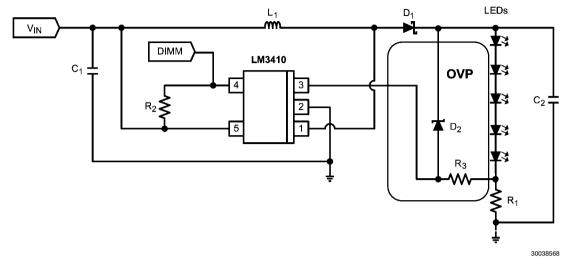
LM3410Y (525kHz): V $_{\rm IN}$  = 2.7V to 5.5V, 5 x 3.3V LEDs, (V $_{\rm OUT}$   $\cong$  16.5V) I $_{\rm LED}$   $\cong$  50mA
