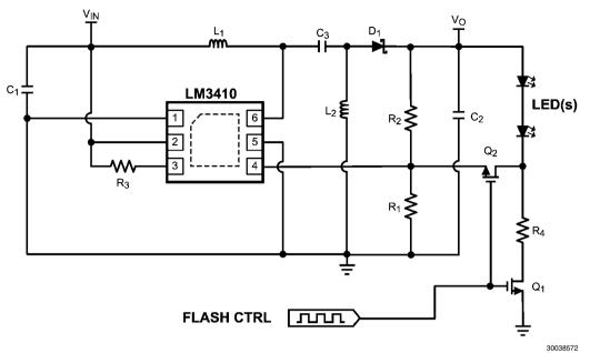
LM3410X (1.6MHz):  $V_{IN}$  = 2.7V to 5.5, ( $V_{OUT}$   $\cong$  7.5V),  $I_{LED}$   $\cong$  1.5A Flash
