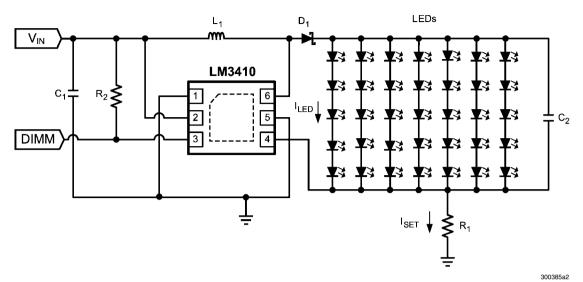
LM3410X (1.6MHz):  $V_{IN}$  = 2.7V to 5.5V, 7 x 5 x 3.3V LEDs, ( $V_{OUT}$   $\cong$  16.7V),  $I_{LED}$   $\cong$  25mA
