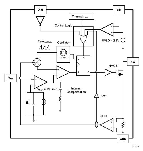
FIGURE 1. Simplified Block Diagram
