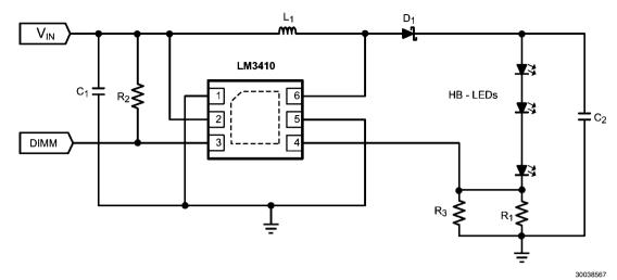
LM3410X (1.6MHz):  $V_{IN}$  = 2.7V to 5.5V, 3 x 3.4V LEDs, ( $V_{OUT}$   $\cong$  11V)  $I_{LED}$   $\cong$  340mA
