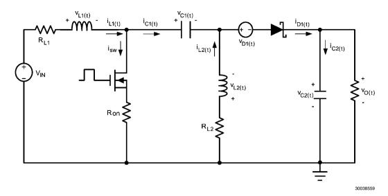
FIGURE 15. SEPIC Simplified Schematic
