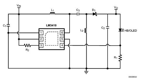
LM3410X (1.6MHz):  $V_{IN}$  = 2.7V to 5.5V, ( $V_{OUT} \approx 3.8V$ )  $I_{LED} \approx 300$ mA
