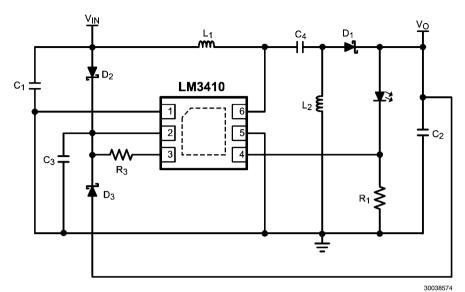
LM3410X (1.6MHz):  $V_{IN}$  = 1.9V to 5.5V,  $V_{IN}$  > 2.3V (TYP) for Start Up
