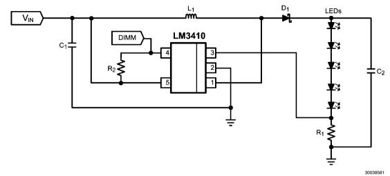
LM3410Y (550kHz): V $_{\rm IN}$  = 2.7V to 5.5V, 5 x 3.3V LEDs, (V $_{\rm OUT}$   $\cong$  16.5V) I $_{\rm LED}$   $\cong$  50mA
