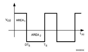
FIGURE 13. Inductor Volt-Sec Balance Waveform
