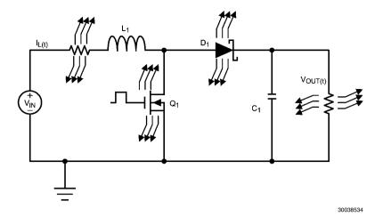
FIGURE 9. Thermal Schematic
