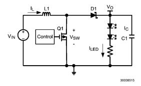
FIGURE 2. Simplified Boost Topology Schematic
