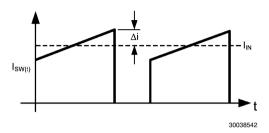
FIGURE 11. LM3410 Switch Current
