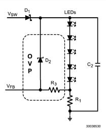
FIGURE 6. Overvoltage Protection Circuit
