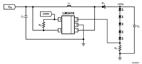
LM3410X (1.6MHz): V $_{\rm IN}$  = 2.7V to 5.5V, 5 x 3.3V LEDs, (V $_{\rm OUT}$   $\cong$  16.5V) I $_{\rm LED}$   $\cong$  50mA
