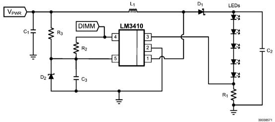
LM3410X (1.6MHz):  $V_{PWR}$  = 9V to 14V, ( $V_{OUT}$   $\cong$  16.5V)  $I_{LED}$   $\cong$  50mA
