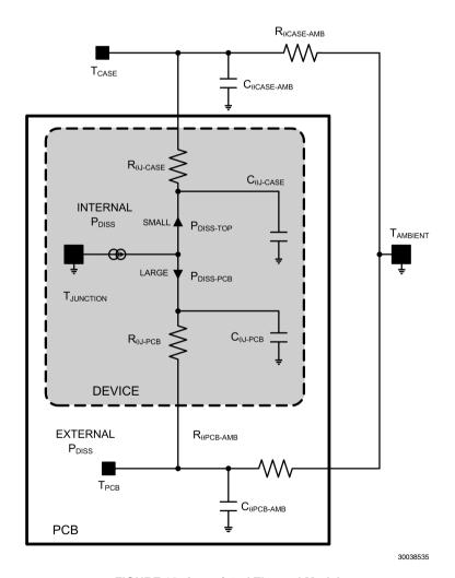
FIGURE 10. Associated Thermal Model
