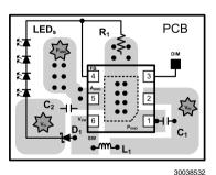
FIGURE 7. Boost PCB Layout Guidelines
