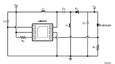
FIGURE 14. HB/OLED SEPIC CONVERTER Schematic
