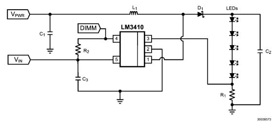
LM3410X (1.6MHz):  $V_{PWR}$  = 9V to 14V,  $V_{IN}$  = 2.7V to 5.5V, ( $V_{OUT}$   $\cong$  14V)  $I_{LED}$   $\cong$  50mA
