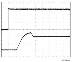
$I_{\rm LED}$  = 1A nominal,  $V_{\rm IN}$  = 12V,  $V_{\rm LED(s)}$  = 20V, no lead compensation Top trace: EN input, 1V/div, DC Bottom trace:  $I_{\rm LED}$ , 500mA/div, DC
