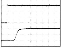
$I_{LED}$  = 1A nominal,  $V_{IN}$  = 12V,  $V_{LED(s)}$  = 20V, with lead compensation Top trace: EN input, 1V/div, DC Bottom trace:  $I_{LED}$ , 500mA/div, DC T = 1ms/div
