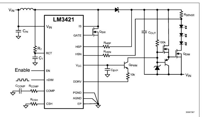
FIGURE 11. LM3421 Buck-Boost (Flyback) Topology with High Speed Dimming
