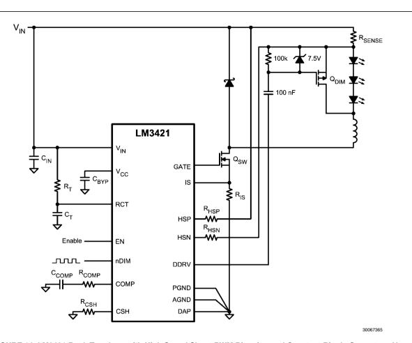
FIGURE 14. LM3421 Buck Topology with High Speed Shunt PWM Dimming and Constant Ripple Current vs.  $V_{\rm IN}$
