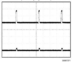
$$\begin{split} &I_{LED}=1\text{A nominal, V}_{IN}=12\text{V, V}_{LED(s)}=20\text{V} \\ &\text{Top trace: nDIM input, 2V/div, DC} \\ &\text{Bottom trace: }I_{LED},500\text{mA/div, DC} \end{split}$$
