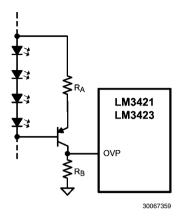
FIGURE 4. LED Forward Voltage OVP Sensing
