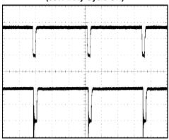
$$\begin{split} & I_{LED} = 1\text{A nominal, V}_{IN} = 12\text{V, V}_{LED(s)} = 20\text{V} \\ & \text{Top trace: nDIM input, 2V/div, DC} \\ & \text{Bottom trace: I}_{LED}, 500\text{mA/div, DC} \end{split}$$
