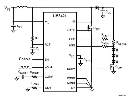
FIGURE 10. LM3421 Boost Topology with High Speed Dimming
