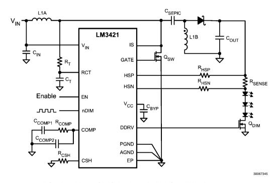
FIGURE 12. LM3421 SEPIC Topology with High Speed Dimming
