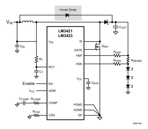
FIGURE 6. Boost Topology with Inrush Diode
