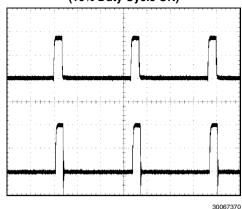
$I_{LED}=1A$  nominal,  $V_{IN}=12V,\ V_{LED(s)}=20V$ Top trace: nDIM input, 2V/div, DC Bottom trace:  $I_{LED}$ , 500mA/div, DC  $T=10\mu s/div$
