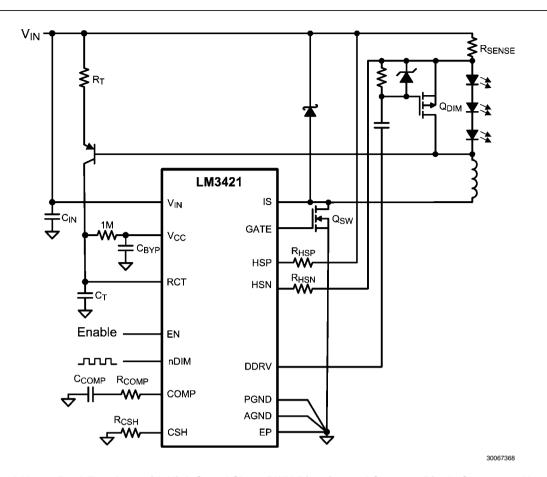
FIGURE 13. LM3421 Buck Topology with High Speed Shunt PWM Dimming and Constant Ripple Current vs.  $V_{\mathsf{LED}}$
