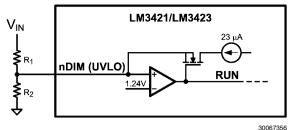
FIGURE 1. Under-Voltage Lock-Out Circuitry
