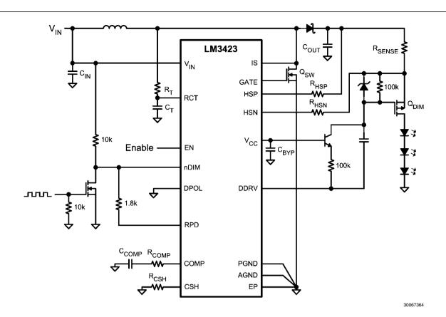
FIGURE 16. LM3423 Boost Topology with High-Side Dimming
