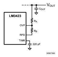
FIGURE 5. OVP Resistive Divider Grounded with RPD
