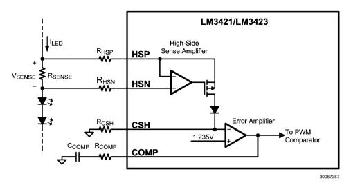
FIGURE 2. LED Current Sense Circuitry
