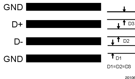
FIGURE 10. Ideal Diode Trace Layout
