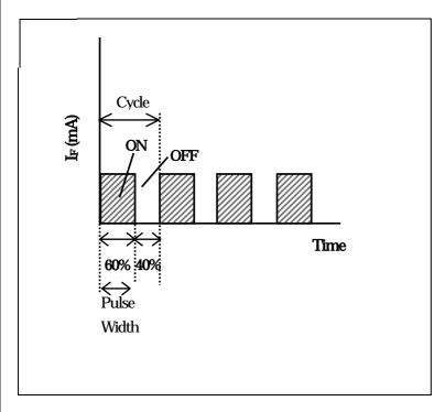
Figure 5: Pulse-width modulation (PWM)
