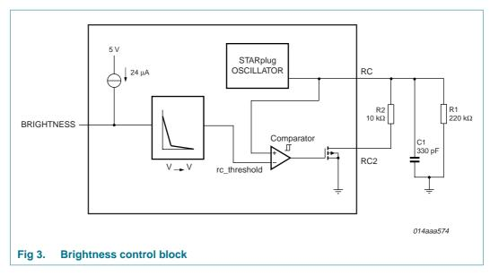
A typical RC waveform is drawn in <u>Figure 4</u>. The RC switch-over threshold is controlled by the BRIGHTNESS pin.
