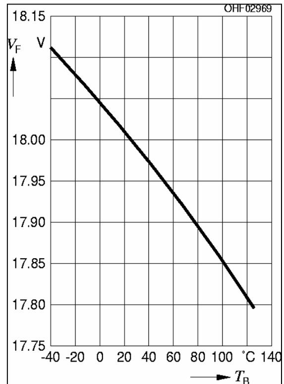
**Figure 9: Typical forward voltage in relation to base plate temperature  $T_B$  ( $I_f = 1 \text{ A}$ ,  $t_p = 10 \text{ ms}$ ).**
