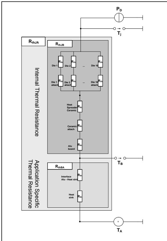
**Figure 13: Equivalent circuit diagram for the thermal resistances.**
