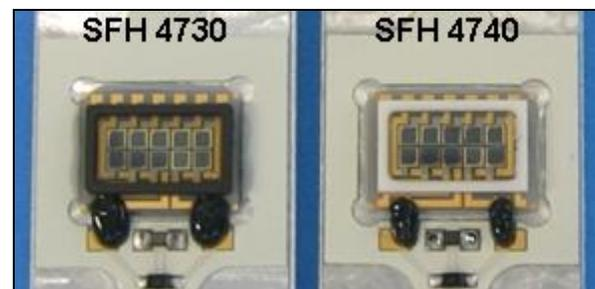
Figure 1: Two frame colours are available for the OSTAR<sup>®</sup>-Observation.
