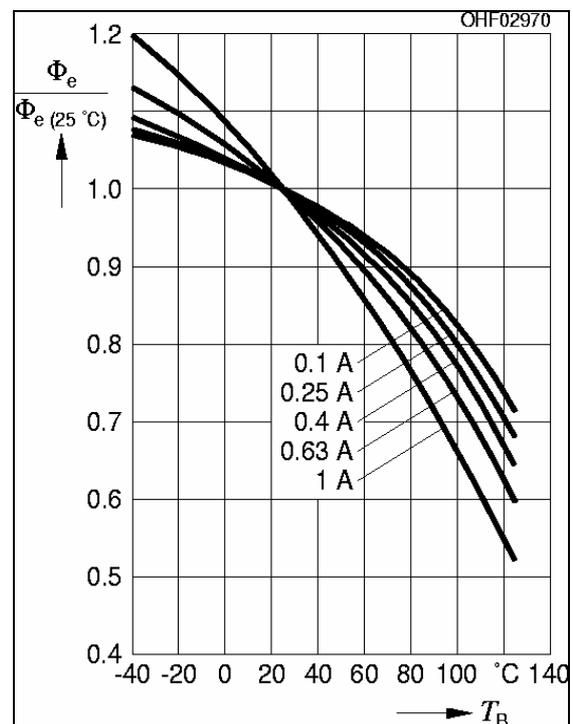
**Figure 10: Relative optical power in relation to base plate temperature for various pulsed currents ( $t_p = 10 \text{ ms}$ ).**
