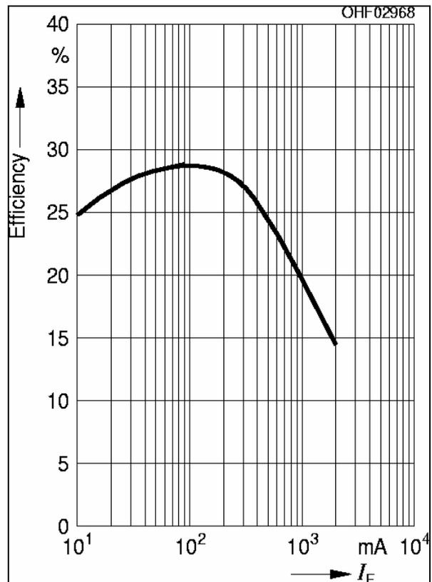
**Figure 8: Efficiency in relation to forward current  $I_f$ ;  $T_B = 25^\circ\text{C}$ ,  $t_p = 100\mu\text{s}$ .**
