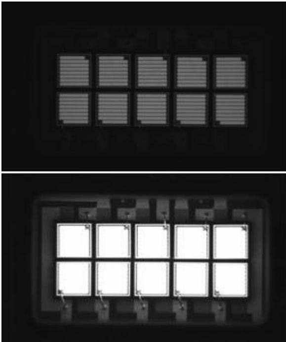
**Figure 6: Radiance images of the OSTAR®-Observation in the near field at very low power (above) and at higher power (below).**
