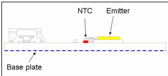
Figure 11: Cross section of the OSTAR®-Observation.
