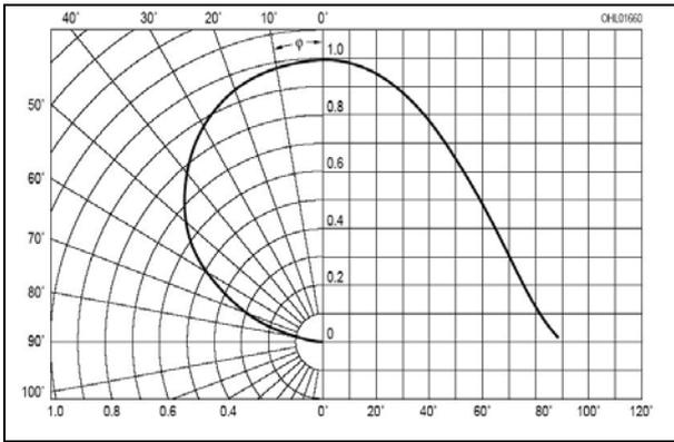
**Figure 5: Radiation characteristics of the OSTAR®-Observation without optics.**
