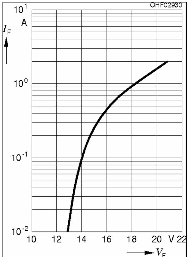
**Figure 7: Current-Voltage characteristic of the OSTAR®-Observation.**
