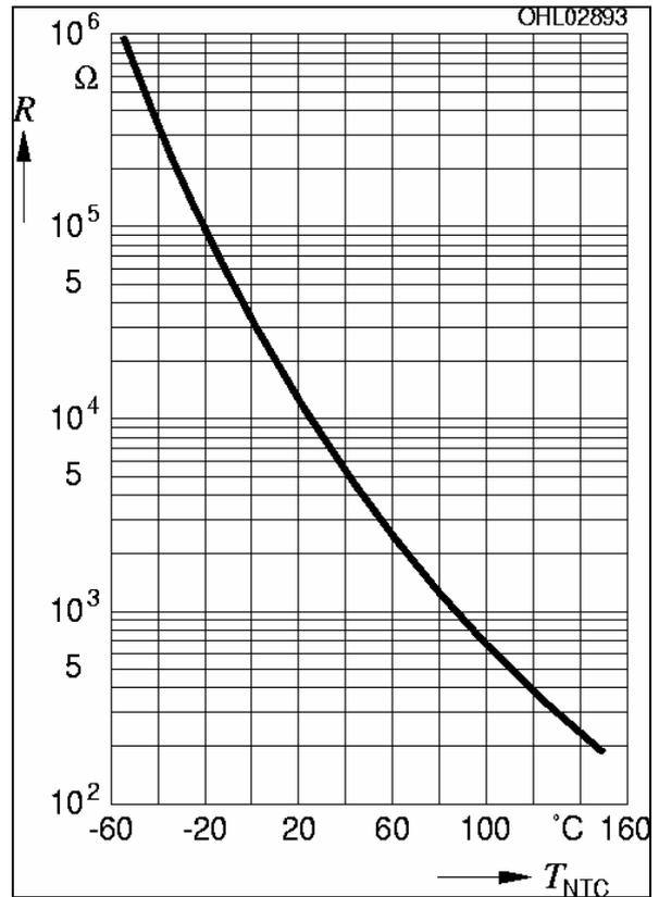
Figure 12: Typical thermistor characteristics for the OSTAR®-Observation (NTC EPCOS 8502).
