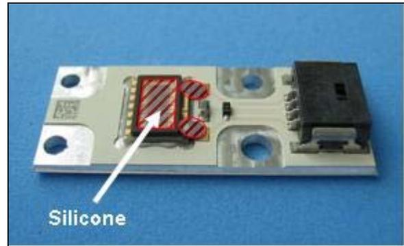
**Figure 2: Areas of the silicone encapsulant of the OSTAR®-Observation (shown in red hatch marks), which must not be damaged.**
