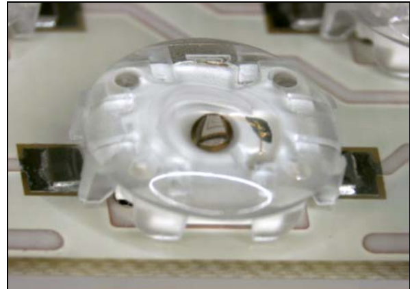
Figure 13: Good solder connection / laser soldering
