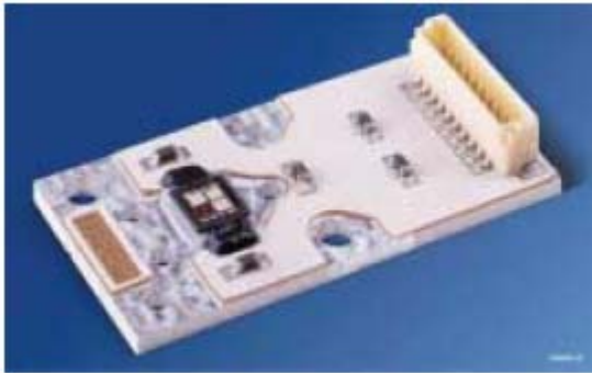
Figure 1: Construction of the OSTAR® Projection
