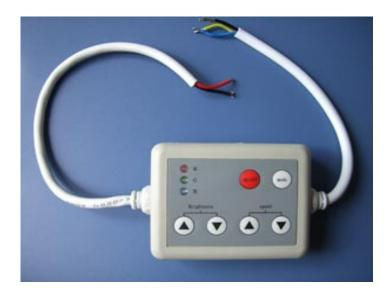
SC-WC2 has all the RGB changing patterns of SC-WC1. It is a small sized controller + dimmer. The dimming patterns is up to 256 levels. Morever it can achieve 100 different color jumpy changing speeds!
