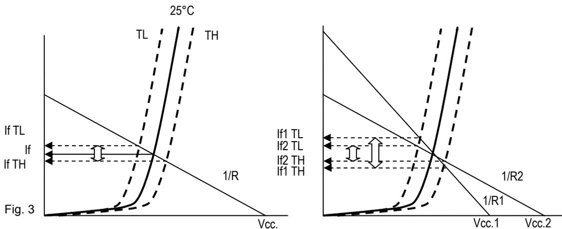
So in a constant voltage circuit, if the supply voltage cannot be set high and there is a large number of LED serial connections relative to the supply voltage so that a large value cannot be obtained for the resistance  $R$ , care is required since the current variations in response to temperature changes and  $V_F$  fluctuations will be larger.
