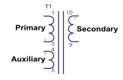
$L_{PRIMARY} = 1.1mH \pm 8\%$ Leakage inductance = 8% of  $L_{PRIMARY}$
