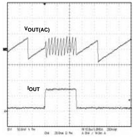
Figure 3. Load Transient Response of the TPS61040 Charge Pump Inverter
