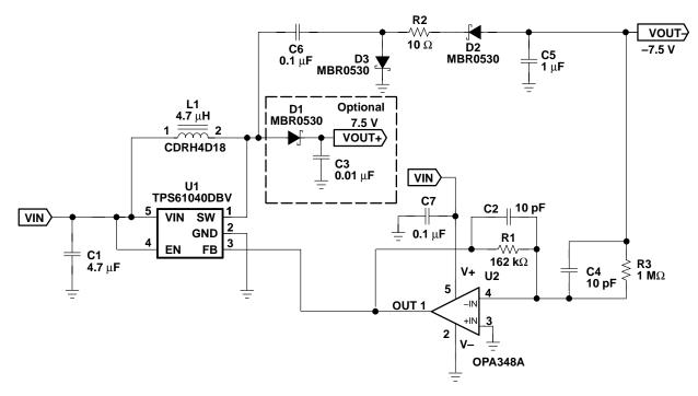
Figure 1. Charge Pump Inverter
