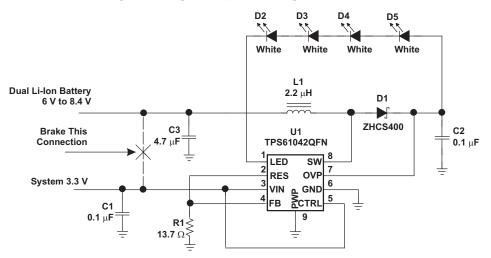
This technique provides two additional benefits: increased efficiency and higher available power output. The following graph shows the increase in efficiency with rising input voltage for a typical four-white-LED application.
