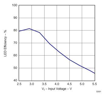
Figure 1. LED Efficiency vs Input Voltage - Torch Mode with ILED=75mA
