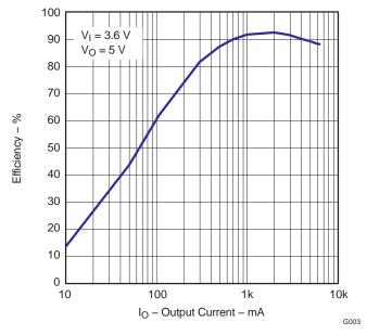
Figure 5. Voltage-Mode Efficiency
