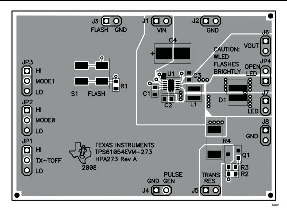
Figure 7. Assembly Layer
