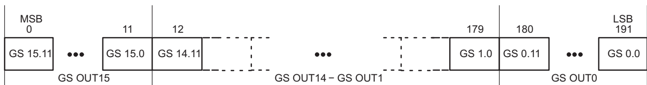
Figure 17. Grayscale Data Packet Format
