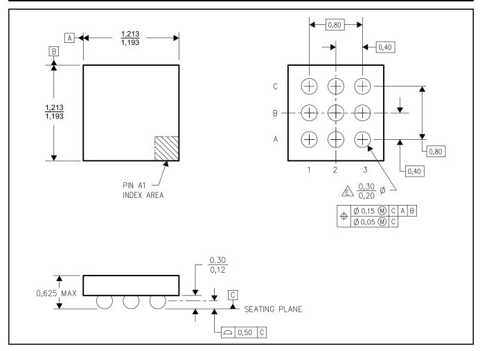
Figure 14. YFF Wafer Chip-Scale Package Dimensions (in mm)
