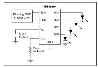
Figure 13. Typical Application Diagram
