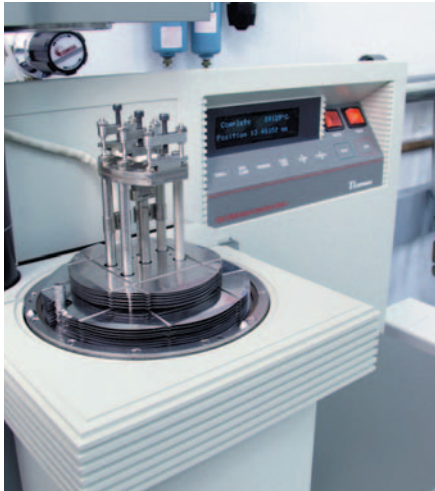
Dynamic Mechanical Analysis (DMA) – Measures the modulus of materials over a range of temperatures.
