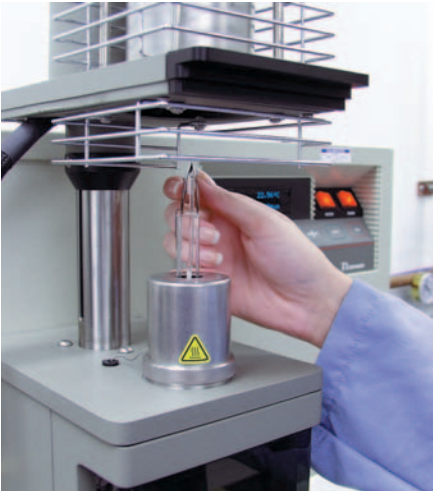
Thermo Gravimetric Analyzer (TGA) – Measures the stability of our dielectrics at high temperatures, baking the materials at prescribed temperatures and measuring weight loss.
