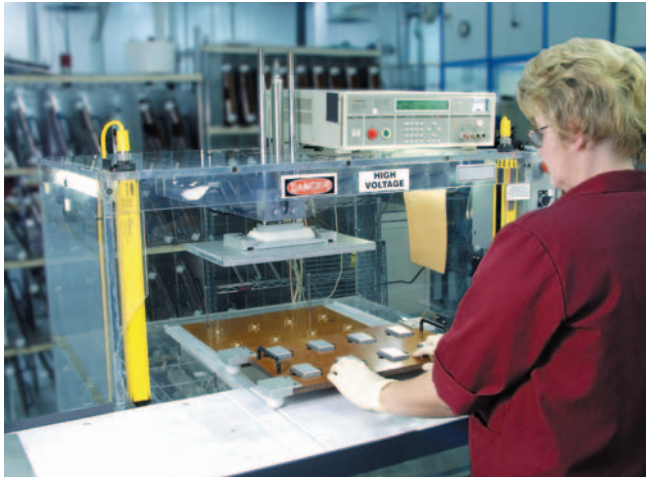
"Proof Test" fixture to test multiple number of finished circuit boards at one time.
