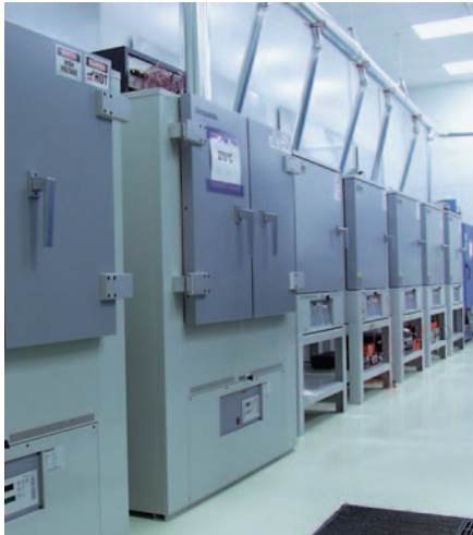
Chamber Ovens – Over 3000 cubic feet of oven capacity is dedicated to long term thermal bias age testing. The ovens take material to temperatures above Tg. At selected intervals, samples are removed and tested to verify material integrity.
