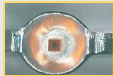
3. LED-Die-Bonding/LED-Die-Bonding
