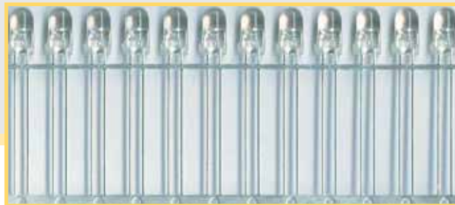
LEDs im Leadframe/ LED in a leadframe
