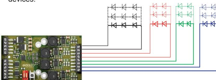
Principle schematic of LED group wiring
