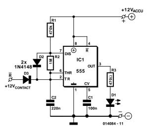
cuit begin to flash. You may then ask what the purpose of D3 is. Well, this has been added in order to prevent the various loads in the car from being connected in parallel with C2 — because that was not the intention, of course.
