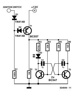
base current will then flow through T1 via D2 and R1, causing T1 to conduct and provide power to the rest of the circuit. This consists of a multivibrator built around T2 and T3, which causes LED D3 to be periodically illuminated. Any desired colour of LED can be used for D3, but the circuit appears quite a bit more modern and effective with a blue LED than with an 'ordinary' red LED.
