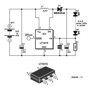
the power switch of the LT1615 can handle larger currents without problems, but the overall efficiency will suffer. Best results will be obtained when  $I_{PEAK}$  is kept well below 700 mA for the LT1615.
