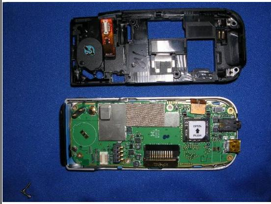
Separate the Upper cover from frame housing
