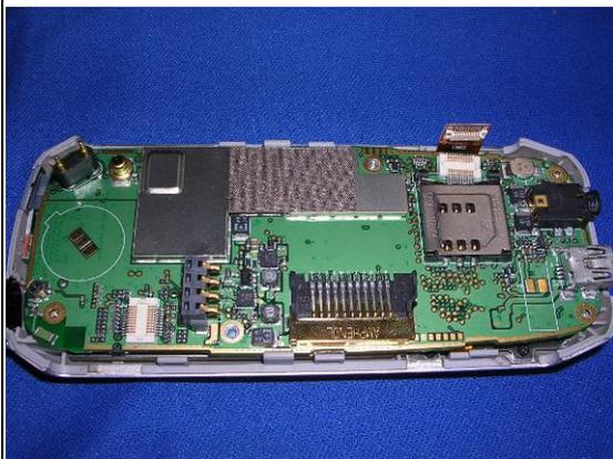
Assemble the MB AND LCD INTO UPPER cover.
