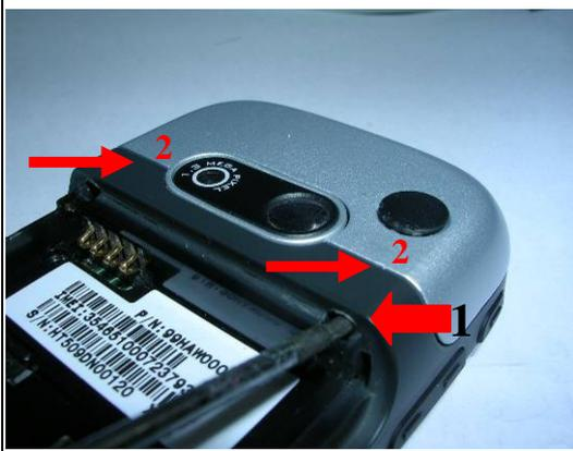
Release the antenna radiator by inserting Precision flat driver type 0.9mm into two holes located at lower part of antenna as shown on picture (1)
