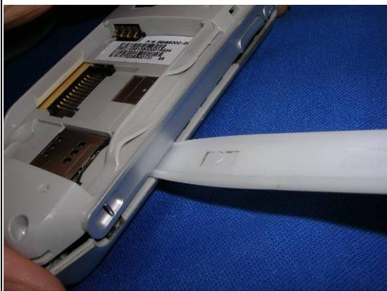
Insert plastic stick into the gap between upper cover and housing to release three hooks which fix them.
