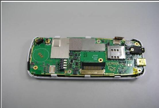
Assemble the switch board connector
