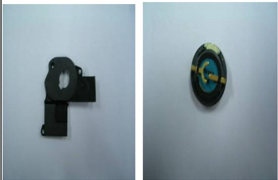
Speaker could be released after removing the sound box cover.
