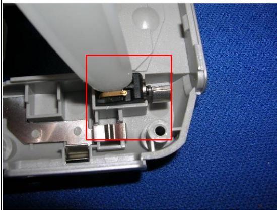
Assembly vibrator into its place on rear cover.
