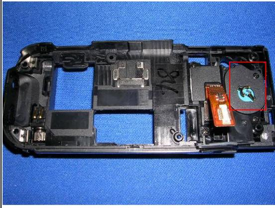
1. Vibrator could be removed from housing.
