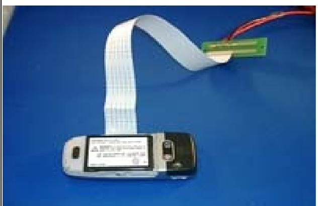
7. Remove original main battery and install battery fixture (E)
