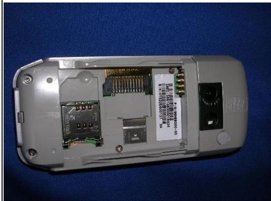
Remove antenna rubber, battery cover, battery from unit
