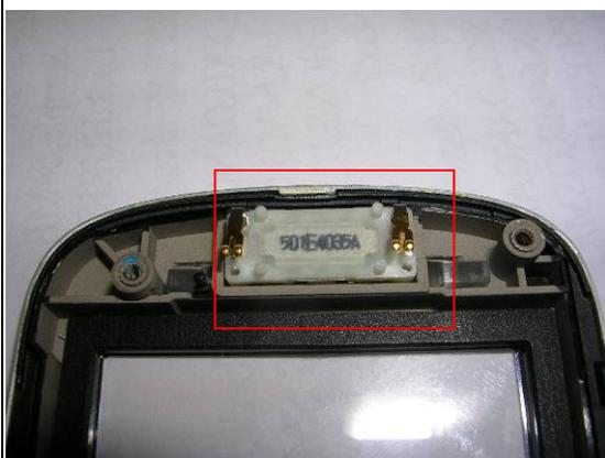
**Assemble** Receiver into its place, notice the two pins **should not bent** on assembly process.
