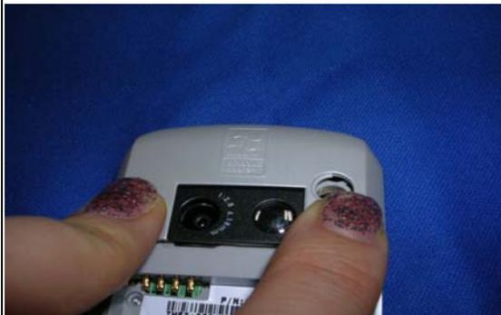
Installed the antenna radiator starting from upper part,
