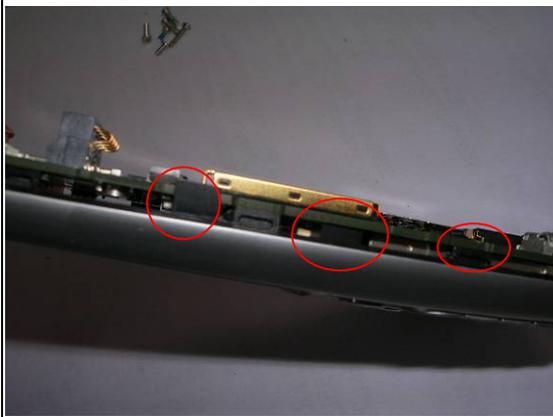
Release 6 hooks which hold the MB with upper cover, starting from left side.
