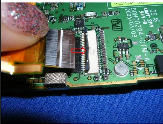
To release the LCD, unlock the connector cover.
