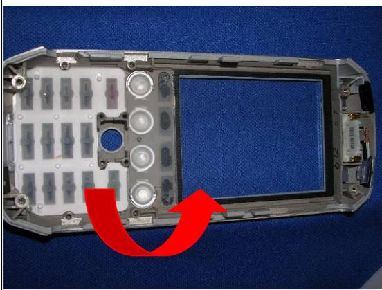
Push out the functional keypad and Numeric keypad from front side
