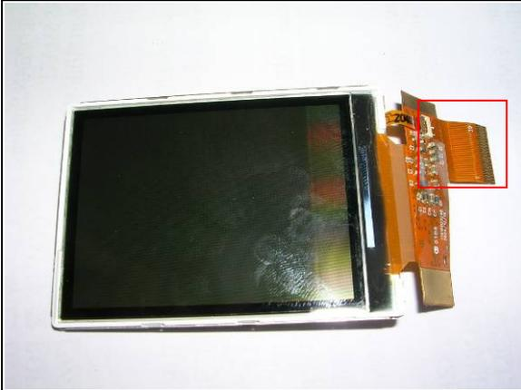
There is a Mylar put on LCD FPC, this Mylar need to be attached when connect the LCD WITH Main board.
