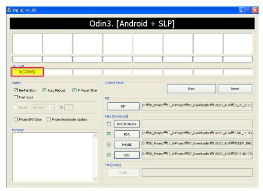
**4**. Start downloading binary file into the device by clicking Start Button on the screen. the green colored "PASS!" sign will appear on the upper-left box if the binary file has been successfully downloaded into the device.
