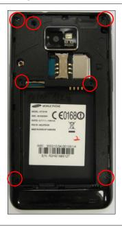
Carefully release the screws at 7 different locations from the rear cover.
