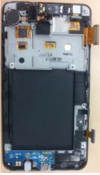
Separate all connector ribbons from the PBA. Separate the PBA from the Front.
