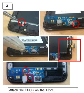
Insert the sub PBA in the hook. Attach the FPCB on the Front. Screw 2 points.(Size: M1.4\*L2) (Torque: 1.1±0.1 kgf.cm)
