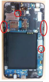
Separate the coaxial cable of antenna assembly from the PBA.
