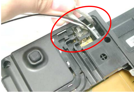
Inverter & camera cable
