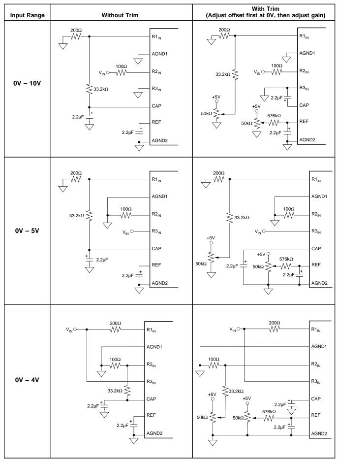
FIGURE 4a. Offset/Gain Circuits for Unipolar Input Ranges.
