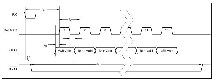
FIGURE 2. Serial Data Timing Using Internal Clock. (CS, EXT/INT and TAG Tied LOW.)
