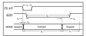
FIGURE 1. Basic Conversion Timing.
