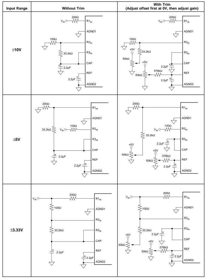
FIGURE 4b. Offset/Gain Circuits for Bipolar Input Ranges.
