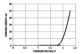
Figure 3. Forward Current vs Forward Voltage
