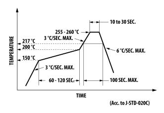
Figure 6. Recommended reflow soldering
