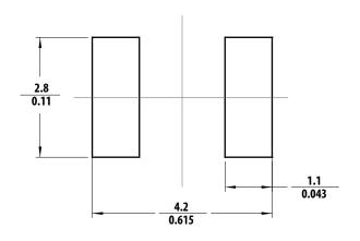
Figure 7. Recommended soldering land pattern
