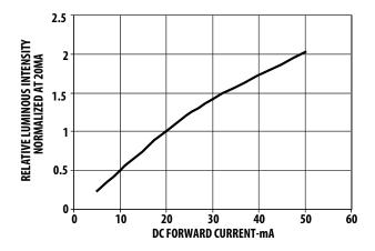
Figure 2. Luminous Intensity vs Forward Current
