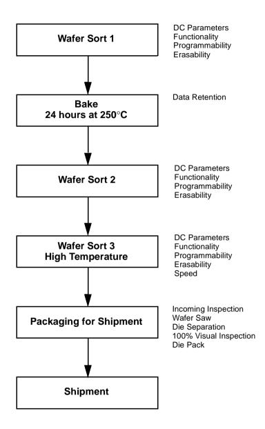
Figure 1. AMD KGD Product Test Flow
