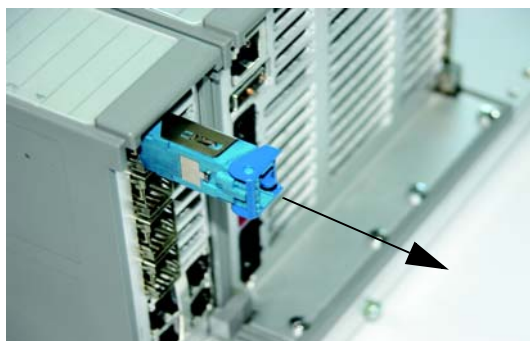
Fig. 21: Disassembling the SFP module
