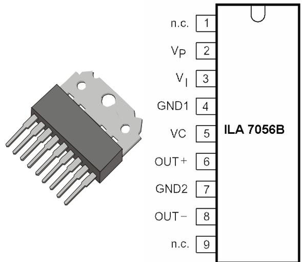
Figure 1. Package and pin connection
