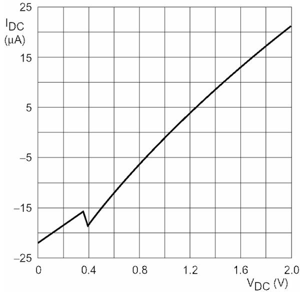
**Figure 5.** Control current as a function of DC volume control.
