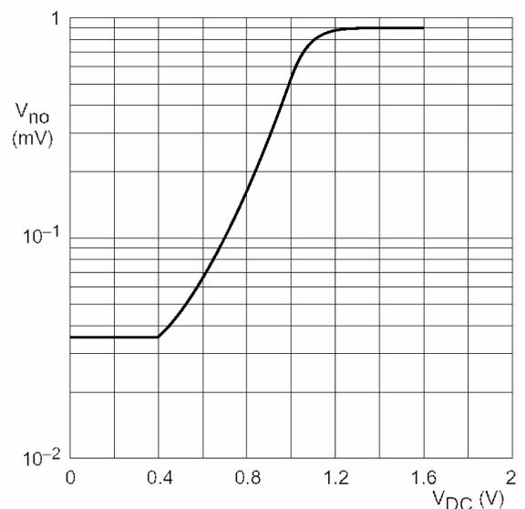
Figure 4. Noise output voltage as a function of DC volume control.
