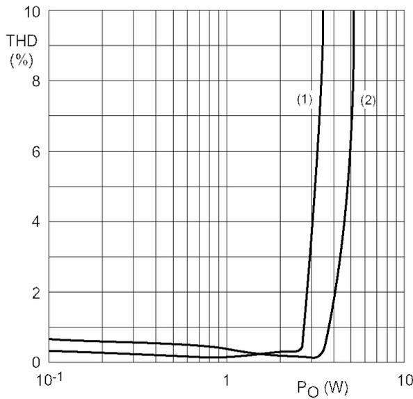
**Figure 7.** Total harmonic distortion versus output power.
