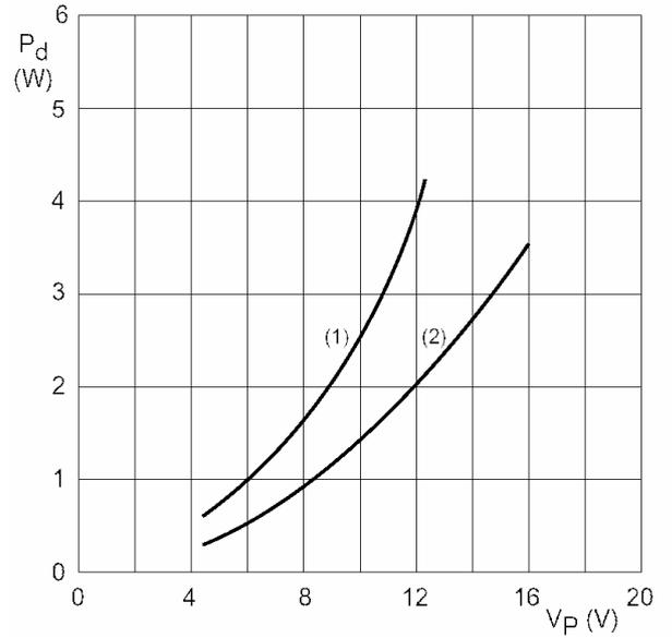
Figure 10. Total worst case power dissipation versus supply voltage.
