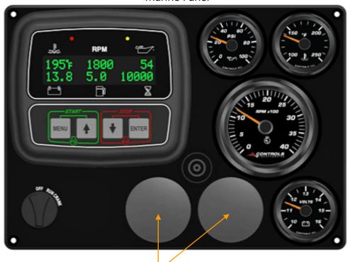
Optional transmission pressure and temperature gauges
