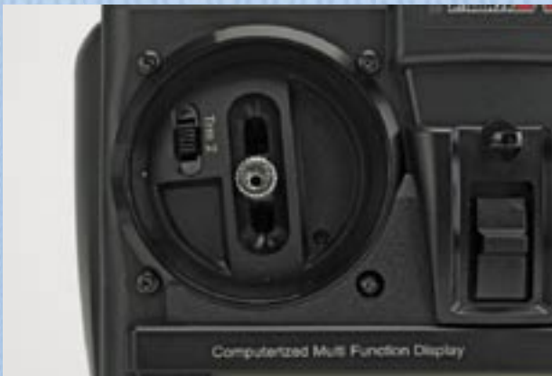
The spring tension, gimball angle and stick height can all be adjusted
