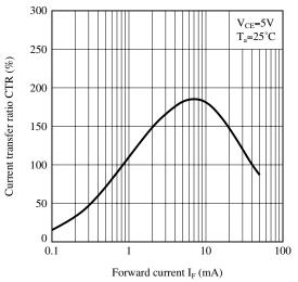
Fig.9 Relative Current Transfer Ratio vs.
