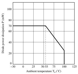
Fig.4 Total Power Dissipation vs. Ambient Temperature
