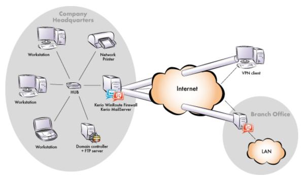
Figure 1.1 Network configuration example
