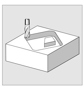
The cycle allows material to be removed with a smaller milling tool. The traversing motions defined by the residual material of the last milling operation and the current tool radius are output in the generated program. The residual material technology can be programmed repeatedly with a succession of decreasing tool radii. No check is made on completion of the cycle for any further residual material in the pocket.
