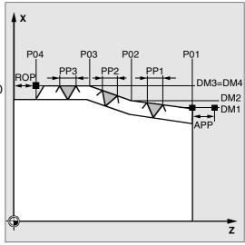
In a second method, the total thread depth is divided into constant infeed depths. The cross-section of cut gets larger from cut to cut. However, if the values for the thread depth are small, this method can create better cutting conditions.
