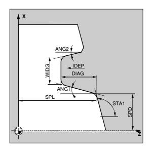
If the programmed groove width is less than the actual tool width, the error message 61602 "Tool width incorrectly defined" is output, the cycle is not started and machining is aborted. The alarm is also output if the value zero has been entered for the tool nose width.
