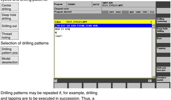
Drilling patterns may be repeated if, for example, drilling and tapping are to be executed in succession. Thus, a name is assigned to the drilling pattern which will later be entered in the screenform "Repeat position".
