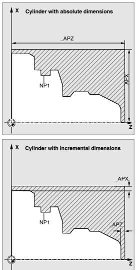
4.10 Extended stock removal cycle - CYCLE950 (SW 5.3 and later)
