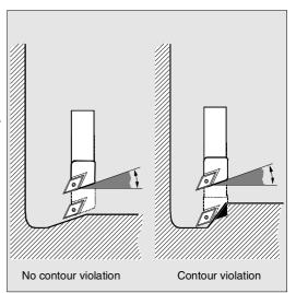
When entering the tool clearance angle, remember that this depends on whether machining is longitudinal or facing. If a tool is to be used for longitudinal and face machining, two tool offsets must be applied if the tool clearance angles are different.
