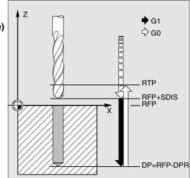
If the values for the reference plane and the retraction plane are identical, a relative depth must not be programmed. The error message 61101 "Reference plane incorrectly defined" is output and the cycle is not executed. This error message is also output if the retraction plane lies behind the reference plane, i.e. the distance to the final drilling depth is smaller.
