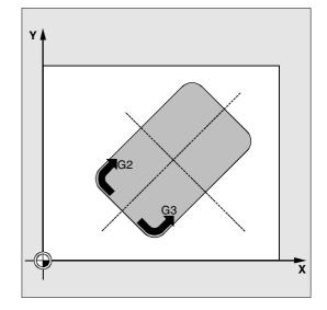
• When machining of the pocket is completed the tool is traversed to the pocket center point on the retraction plane and the cycle is terminated.
