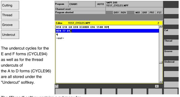
The "Thread" softkey contains a submenu for selecting between single thread cutting or thread chaining.
