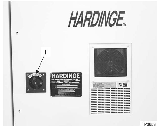
Figure 1.4 - Main Disconnect Switch
