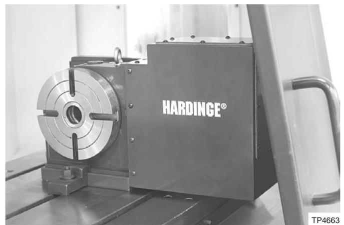
Figure 1.7 - Rotary Table Mounted on the Machine Table
