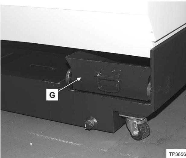
Figure 2.3 - Left Side Chip Pan
