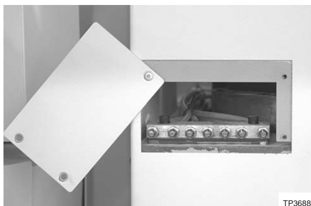
Figure 4.1 - Z Axis Grease Fittings at Front of Tower
