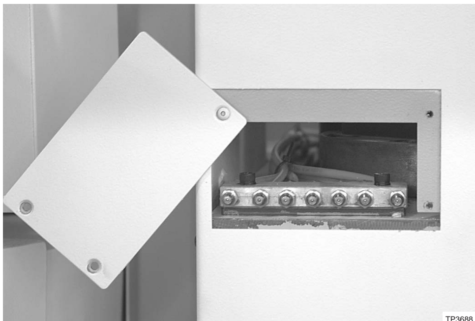
Figure A2.5 - Z Axis Grease Nipple Block
