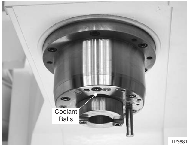
Figure 3.4 - Spindle Face
