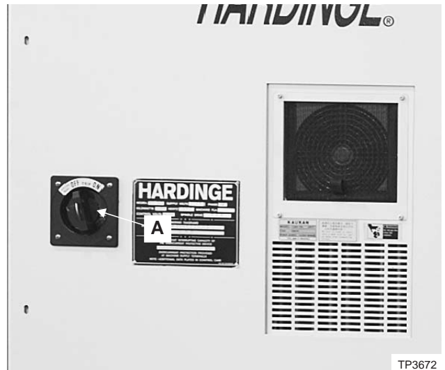
Figure 1.1 - Main Disconnect Switch
