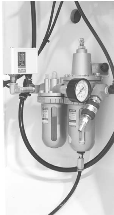
Figure A2.16 - Air Control Assembly Mounted Near the Right Side of the Power Case and on the Side of the Tower (VMC800II through VMC1500II Machines)
