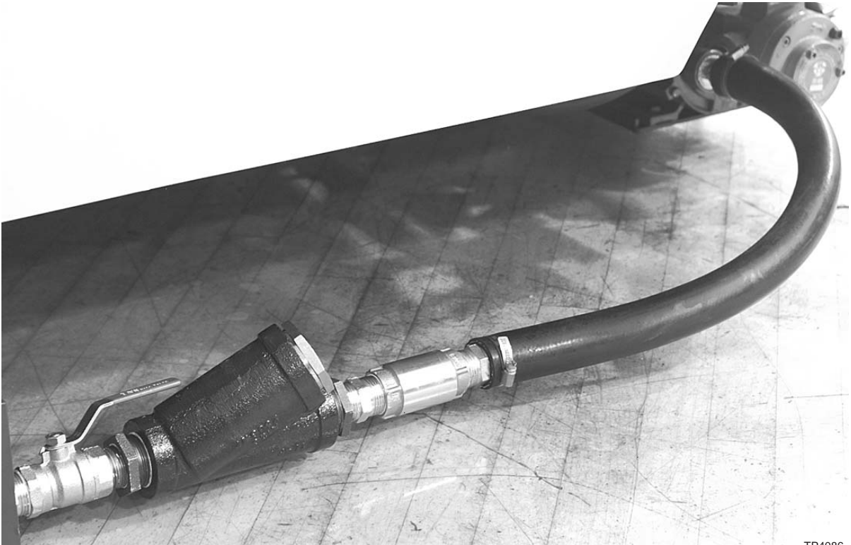
Figure A2.14 - In-Line "Y" Filter and Valves
