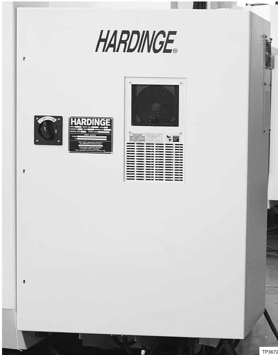
Figure A2.9 - Outside Power Case Door and Heat Exchanger on Standard Machines
