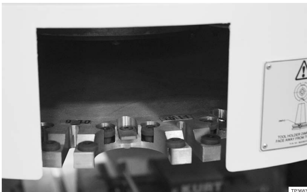
Figure A2.2 - Tool Station (some numbers are on top, other numbers are on the edge or bottom)
