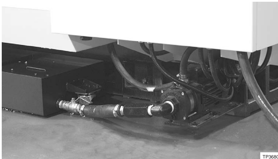
Figure A2.13 - Coolant Pump Under Power Case
