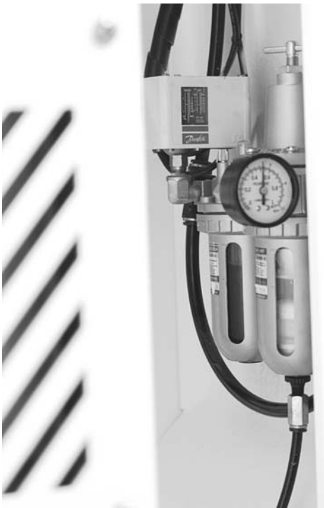
Figure 2.1 - Air Filter/Regulator and Lubricator (VMC600 II Machining Center)
