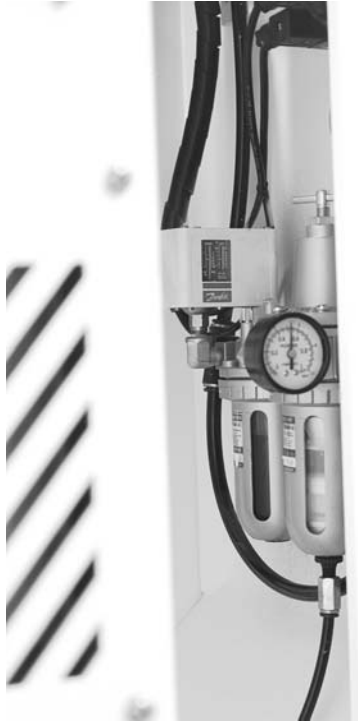
Figure A2.15 - Air Control Assembly Behind Power Case and Mounted on the Side of the Tower (VMC600II Machine)
