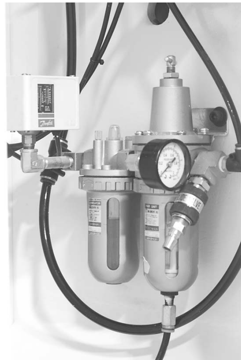
Figure 2.2 - Air Filter/Regulator and Lubricator (All other Series II Machining Centers)
