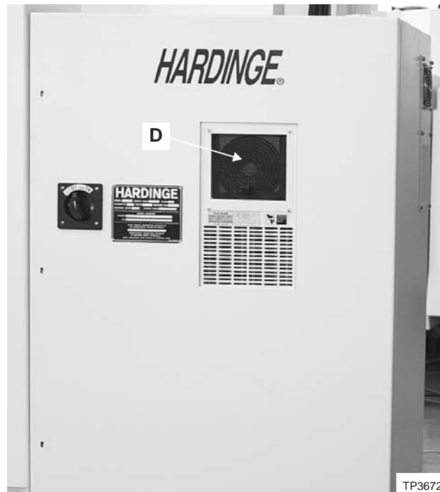
Figure 5.4 - Air Filter on Heat Exchanger
