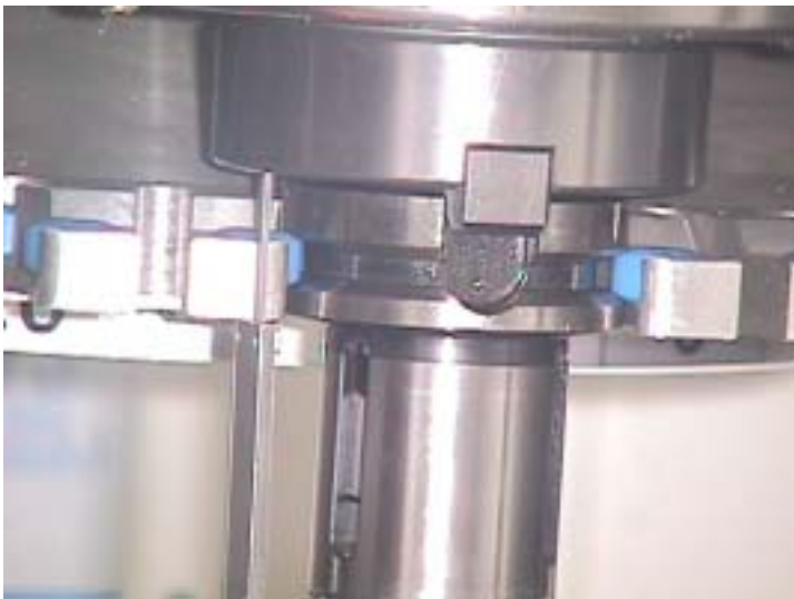
25.To measure below spindle to bottom drum and make a record. 26.Key-in M71 for Drum back position
