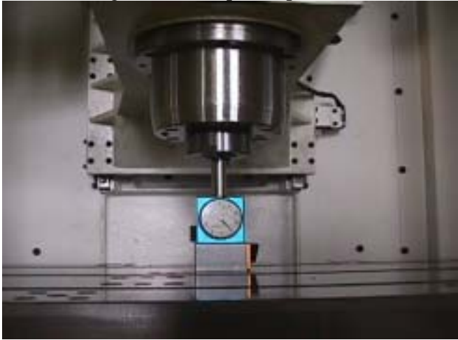
18. To setting table with spindle point
