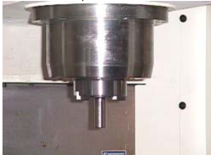
17. To put height gage on the table and length toolholder in to the spindle
