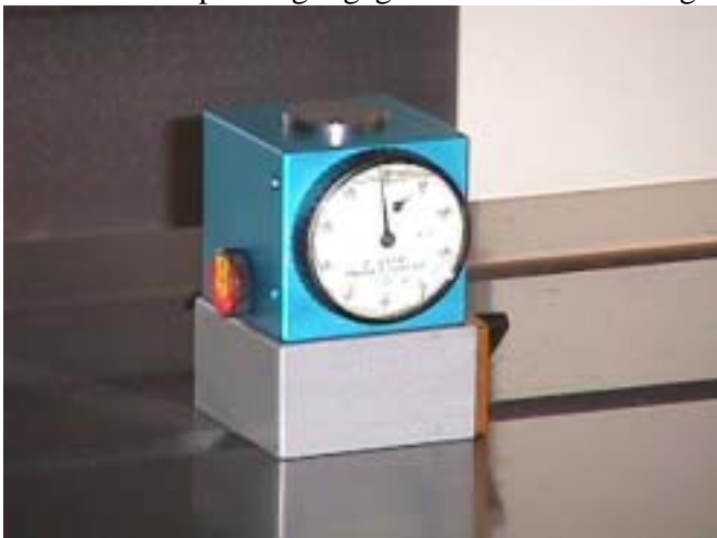
17. To put height gage on the table and length toolholder in to the spindle
