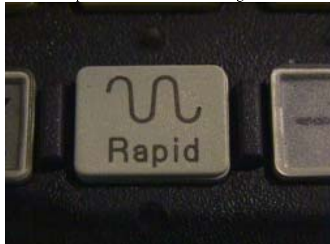
6. Press Rapid Button For Arm 60 Degree
