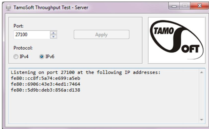
The picture above illustrates the use of the IPv6 protocol. The log window displays the IPv4 or IPv6 addresses used for listening by the application.
