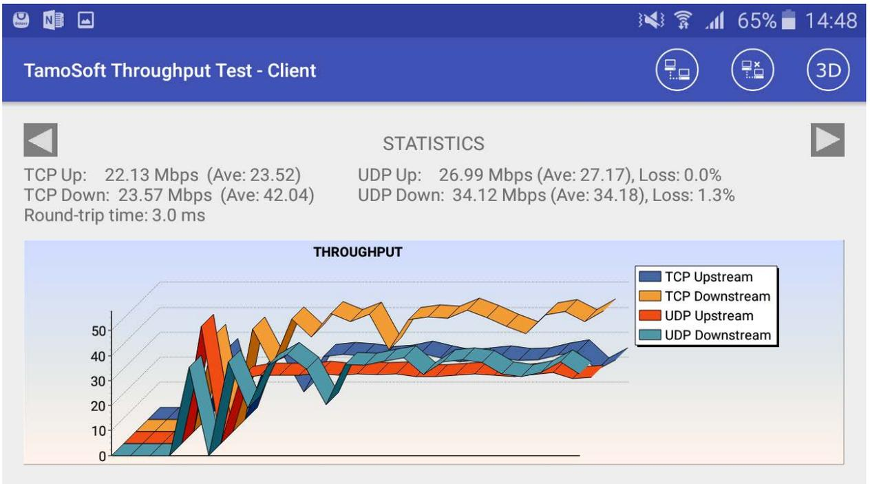
Swipe the chart to switch between Throughput, Loss, and RTT views. Click the **3D** button on the tool bar to toggle the 3D view on and off.
